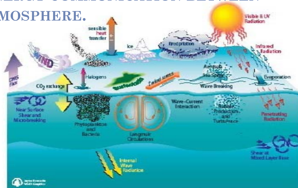
Figure H-7: Schematic of the air-sea interface with dominant processes and fluxes. ORCA aims to significantly improve parameterization of air-sea exchange processes, thus allowing more accurate estimations of regional and global flux fields, and their spatial and temporal variability.
