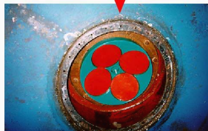
Transducer of bottom mounted ADCP
